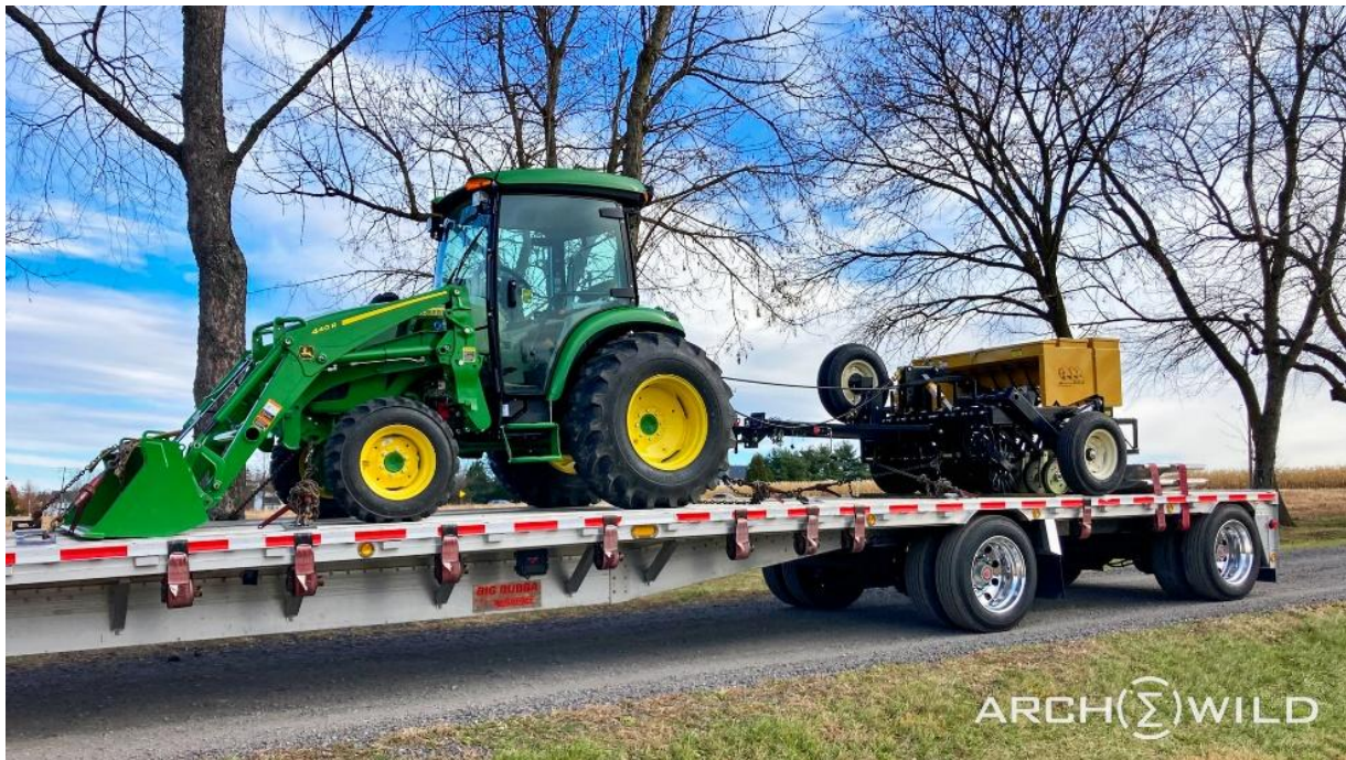
Figure 51 - Tractor and seeder properly loaded and secured on a flatbed.
