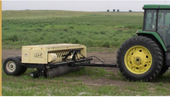
Figure 43 - Specialized broadcast seeders simulate the natural falling and settling of seed and can help prevent planting too deeply
