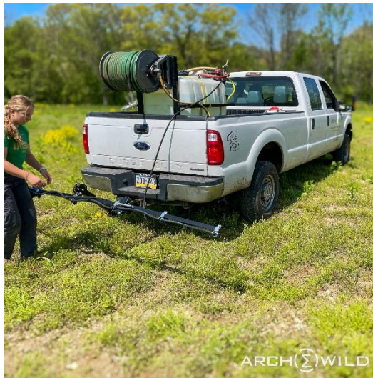
Figure 45 - Technician setting up a truck-mounted boom sprayer
