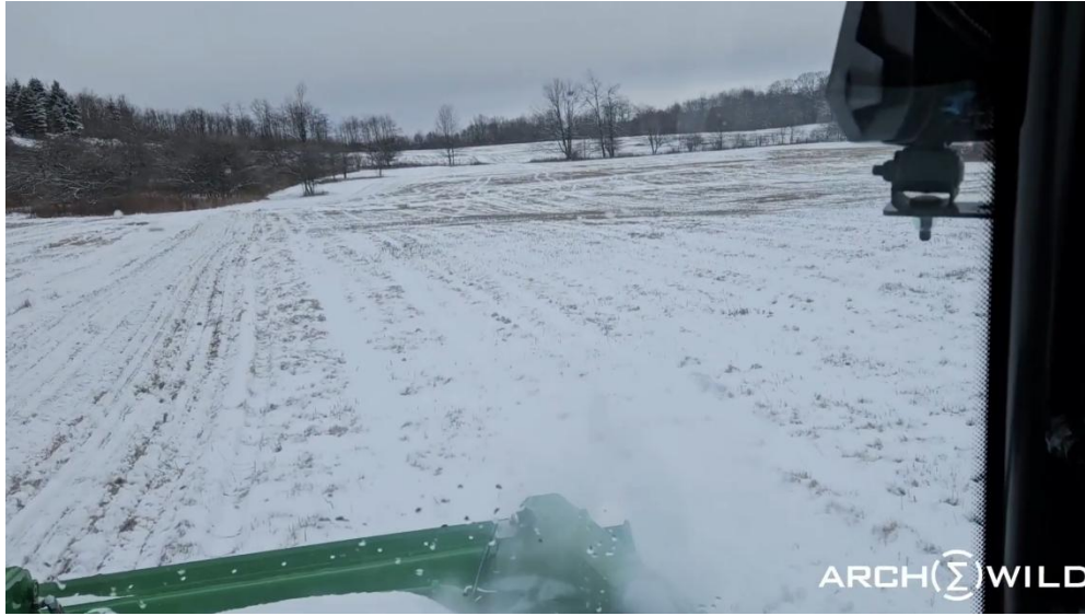
Figure 54 - View from inside a tractor while seeding. Stop, get out, and check the operation of the seeder, and your seed drop rate, about every 30 minutes
