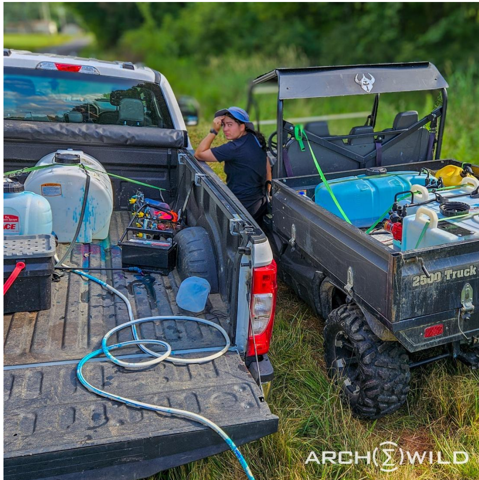
Figure 34 - Low-volume, low-pressure setup for spot treating large meadows in remote locations
