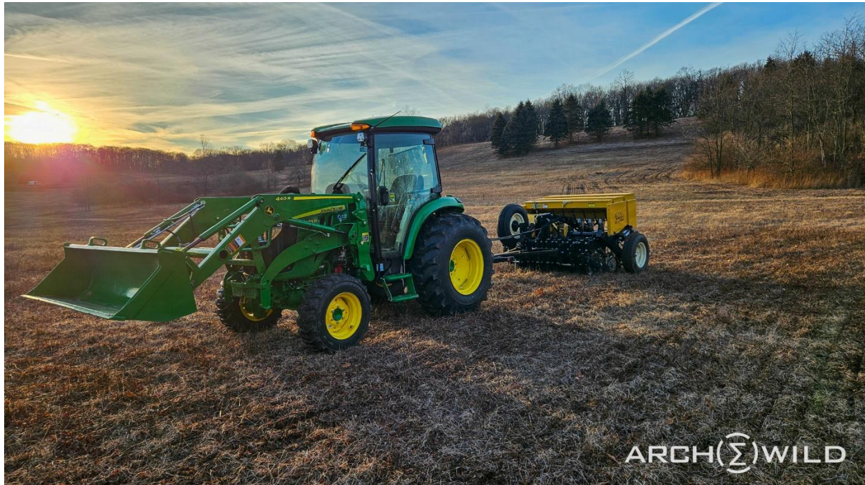
Figure 35 - Steep slopes, soggy areas, groundhog holes, rocks, excessive organic matter, logs, trees, and fences are just some of the challenges facing a seed drill operator. Always thoroughly walk your meadow site before transporting and deploying your seeding equipment
